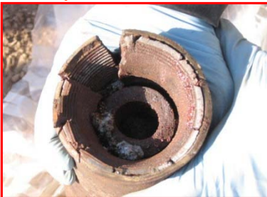
Example - Central burster charge visible
